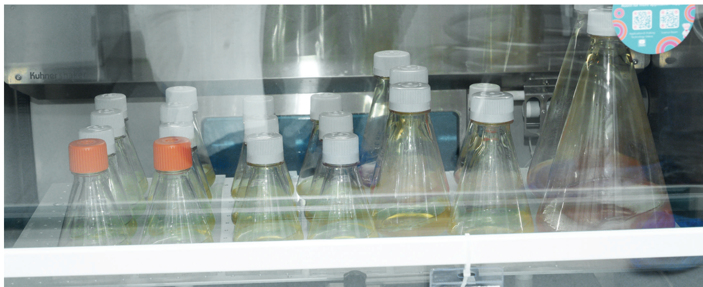
Figure 3: Cell-Specific Perfusion Rate (CSPR) screening at shake flask scale. CSPR between 20-30 (pL/cell/day) was ideal for this process.
